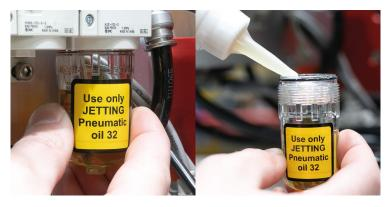
**Alternative 2.** Unscrew the entire container by hand counterclockwise and pour the oil directly into the container.
