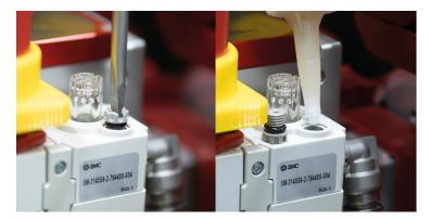
Alternative 1. Loosen the oil container screw and fill.
